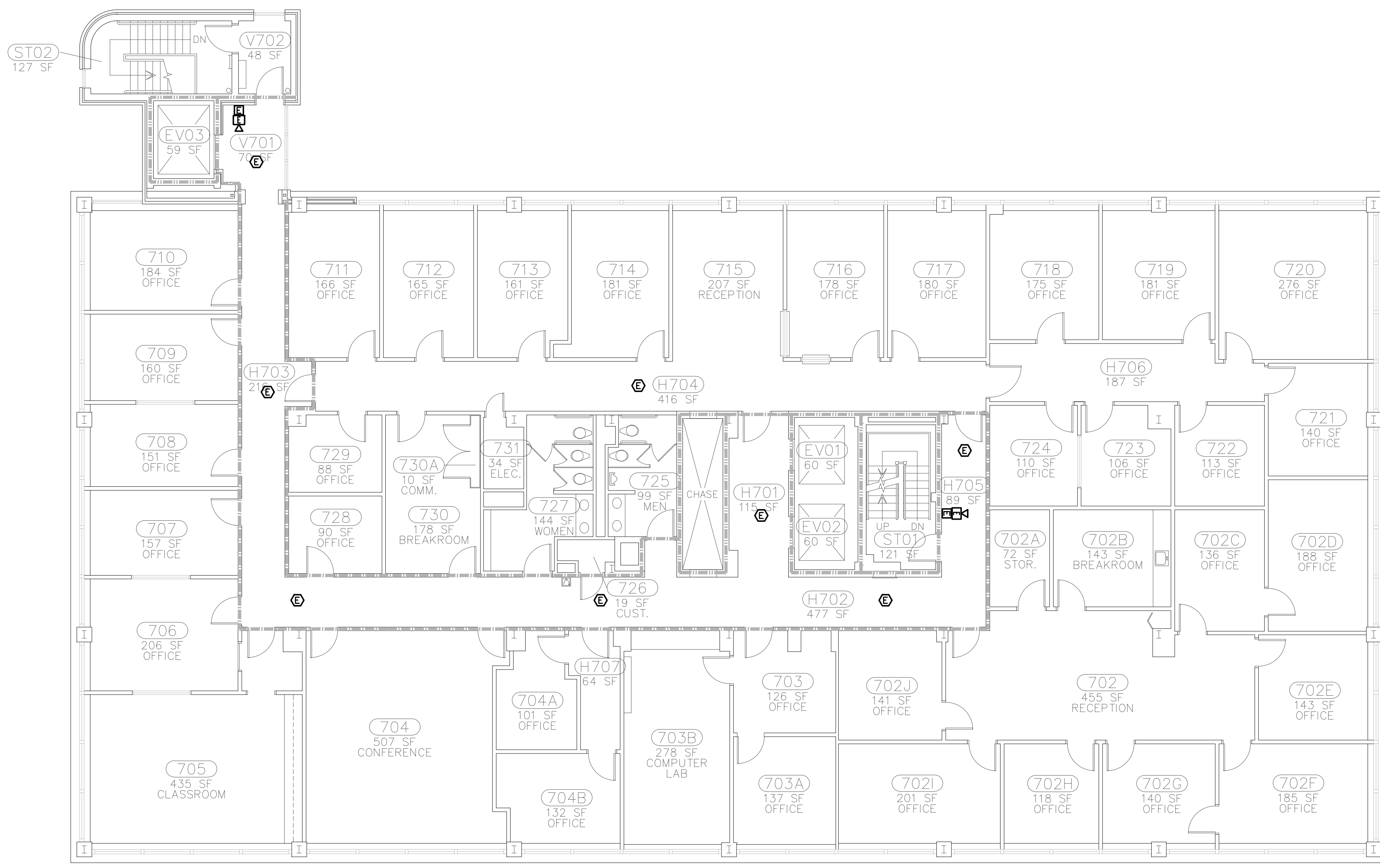
FIRE ALARM - SEVENTH FLOOR DEMOLITION SCALE: 1/8"=1'-0"
